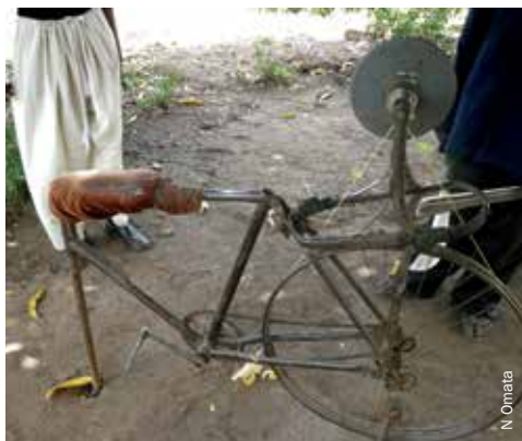
Modified bike for sharpening farm tools in Nakivale.
